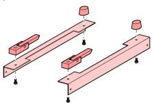
Turn over the TPG 300 and fix both angle profiles to the TPG 300 side panels as shown.
