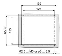
For reducing the mechanical strain on the front panel, preferably support the unit.
