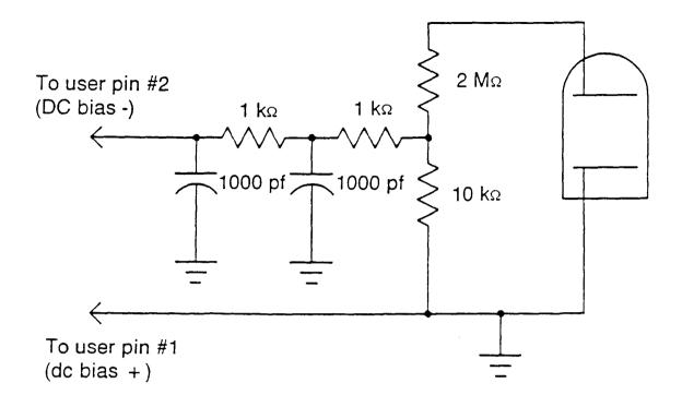
Figure 1. DIVIDER/FILTER CONFIGURATION
